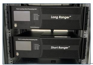
The SHORT RANGER™ system can be employed for real-time, precise detection and location of perimeter security threats on fences, walls or other types of perimeter barriers. The core Ranger™ technology acts as a continuous microphone designed to "monitor" over a quasi-DC to 500 kHz bandwidth, to very distinctive frequencies and energy profiles generated by intrusion events, while discriminating between normal and ambient conditions.
