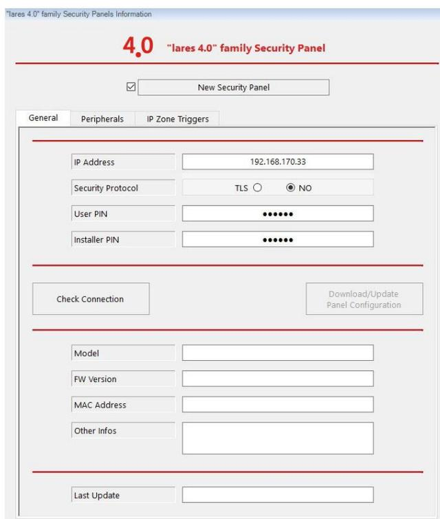
After entering the parameters, you can check the reachability of the new Security Panel using the "Check Connection" button. If everything is OK, the fields below the button used will be filled.
