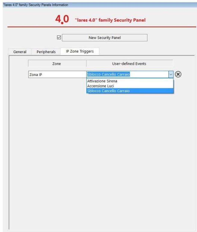
In the previous example, 3 User Events were defined, respectively “Attivazione Sirena” (Siren Activation), “Accensione Luci” (Turning on the Lights) and “Sblocco Cancello Carraio” (Driveway Gate Unlock); the latter is assigned as a Trigger to the only IP Zone present.
