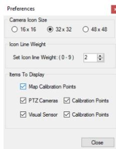
**Camera Icon Size** sets the size of the icon on the map **and Icon Line Weight** sets the length weight between camera icon and camera calibration point icon.
