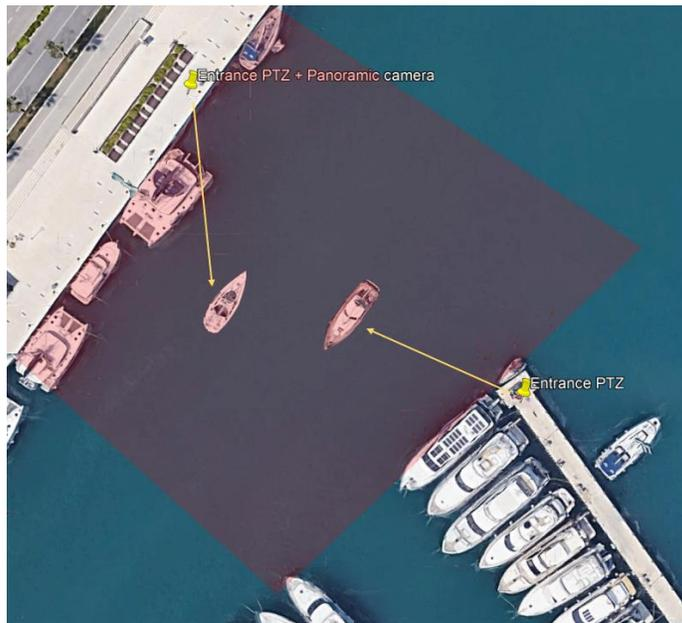
Distance from each PTZ camera to each boat is calculated and minimum distance criteria is applied.
