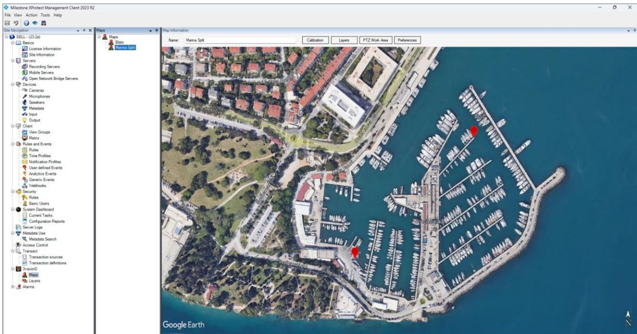
After map calibration, cameras are calibrated with similar procedure. Based upon type of the camera, there are two different calibration procedures, one is for PTZ cameras and other one is for “Non-moving” cameras (Dome, Bullet, etc).
