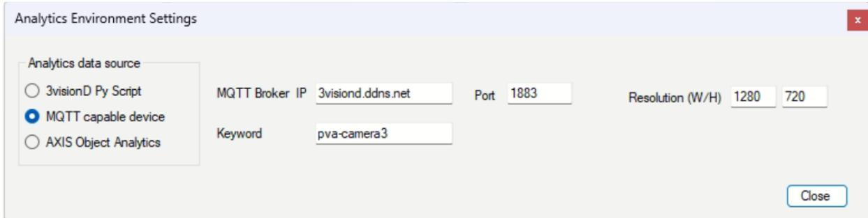
MQTT Broker IP, Port and Keyword are the MQTT settings and the Resolution is the image resolution set as CVEDIA parameter. Image below shows one example of CVEDIA configuration. Axis camera with configuration string that sets camera 3 resolution to 1280x720.
