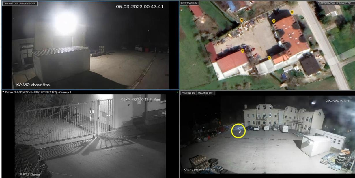
Live map is displaying each camera location and camera type is displayed in XProtect Smart Client upper right corner. Both dome and panoramic camera are set to control PTZ camera.
