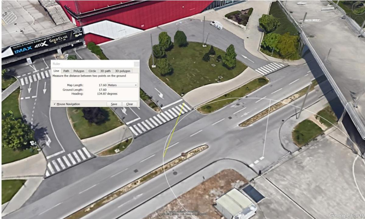
Location of video stream centre point is intersection point of circle a line when line has length of 17.6 m. Inserting placemark in this position will defined geo coordinates for video stream centre point.
