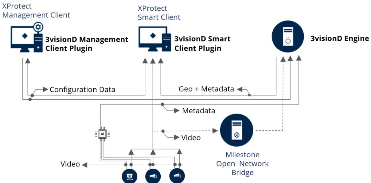
**3visionD Management Client plugin** is used for system configuration. It contains maps and cameras configuration data as well as definitions of layers and their functionalities. 3visionD Smart Client Plugin and 3visionD Engine module are accessing configuration data from this plugin.
