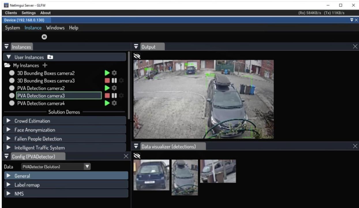
Based upon detected object, automated PTZ camera tracking is activated and PTZ camera direction, zoom level and target height are automatically controlled based upon configuration data from 3visionD Management Client Plugin. Depending on the configuration, object can be tracked with one or several PTZ cameras. Furthermore, in
