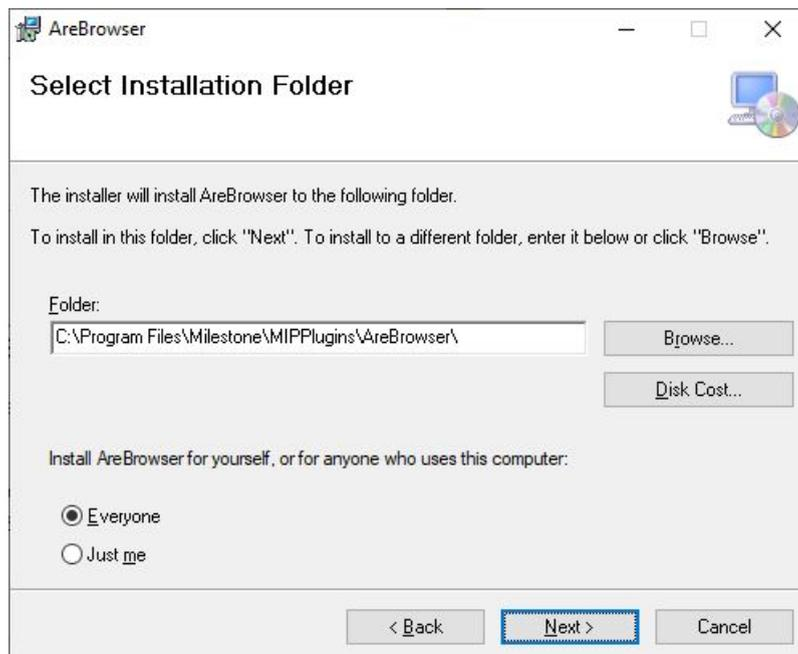
Select the folder where you want to install the AreBrowser plug-in. By default it's "C:\Program Files\Milestone\MIPPlugins\AreBrowser". As specified in the Milestone documentation, to work correctly a plugin must be installed in your "MIPPlugins" directory.
