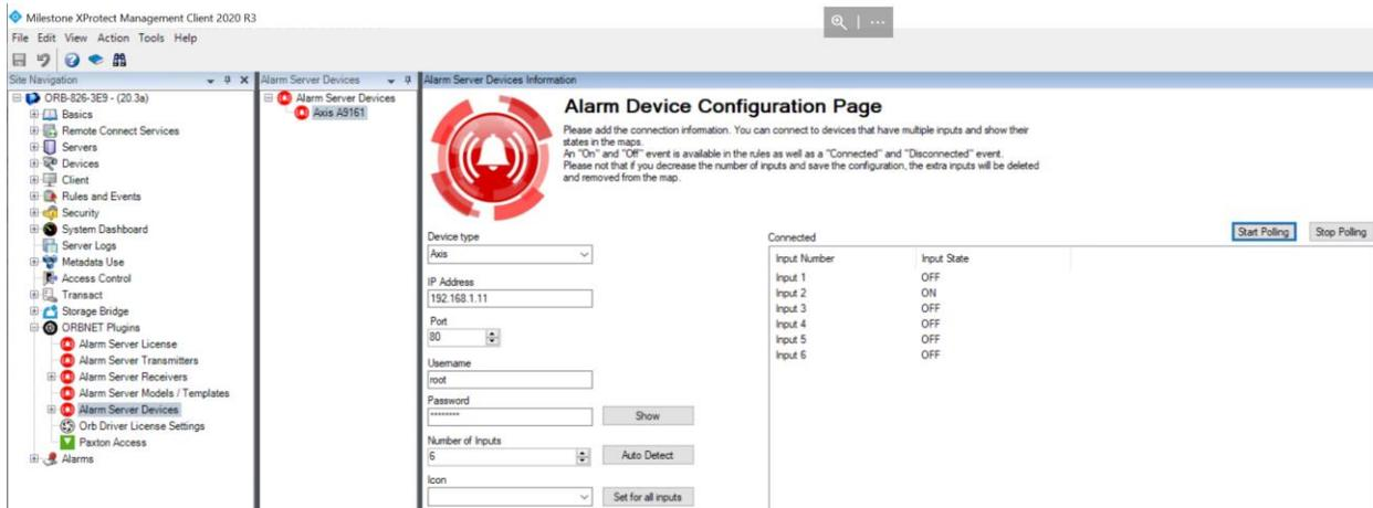
Select the Device type, Set the IP Address, specify the port, username, and password. If successfully connected with the Auto Detect button and the Alarm Server will query the device and then place the inputs in the right window.
