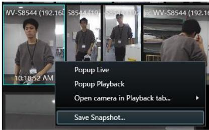
This snapshot is taken directly from the Active Guard server, provided as the Best Shot image. This image is cropped based on the capture object.
