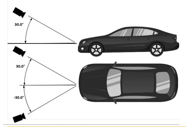
The image of the license plate should not tilt more than 5° horizontally. If the image is tilted more than 5°, we recommended to adjust the camera so that the license plate is displayed horizontally in the live stream.
