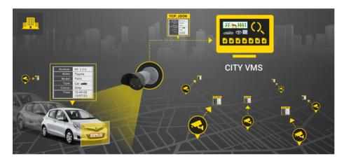
Recognized data from CAMMRA is also sent to municipal VMS, which controls the entire urban video surveillance system. The data received from CAMMRA via TCP protocol are sent to the VMS event engine, where notification messages are generated and the video is searched by vehicle number, color, make and model.
