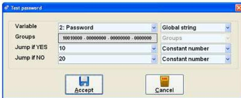
After a failed validation, the system puts in local string 10 (the last local string) a message explaining the reason of the failure.
