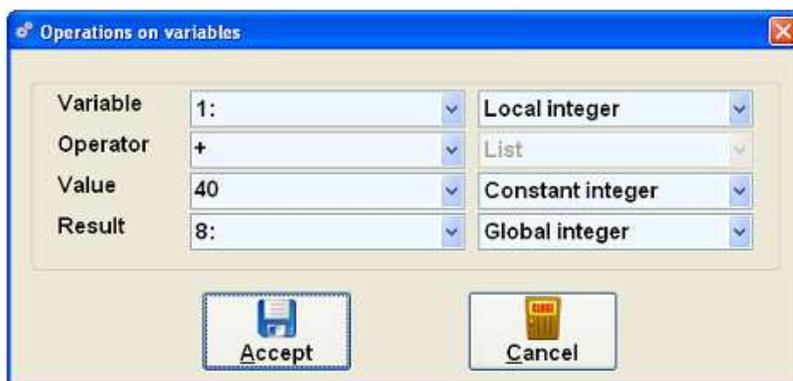
If Value is a numeric value, the operator behaves as if Variable is numeric also, applying a conversion if necessary.
