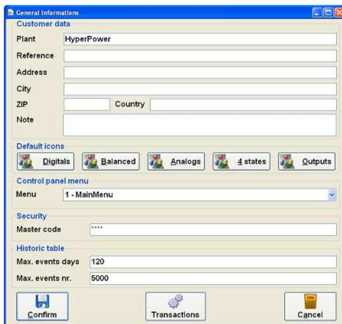
With *Default Icons* section can set the standard icons for graphic representation of digital sensors (status on / off), balanced sensors (on / off / tamper) and outputs (on / off).
