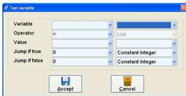
If the variables are of different type (one numeric, one string), the string one is converted in numeric before to execute the numeric test. Conversion of non-numeric strings returns the value 0. If both variables are string, a lexicographical comparison is executed. Upper case and lower case are considered different.
