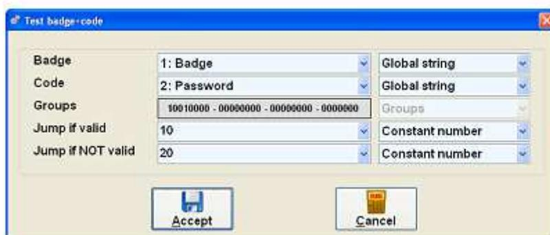
After a failed validation, the system puts in local string 10 (the last local string) a message explaining the reason of the failure.
