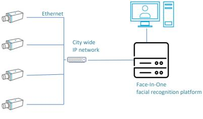
IP Camera or Face capture camera deployed in different city area
