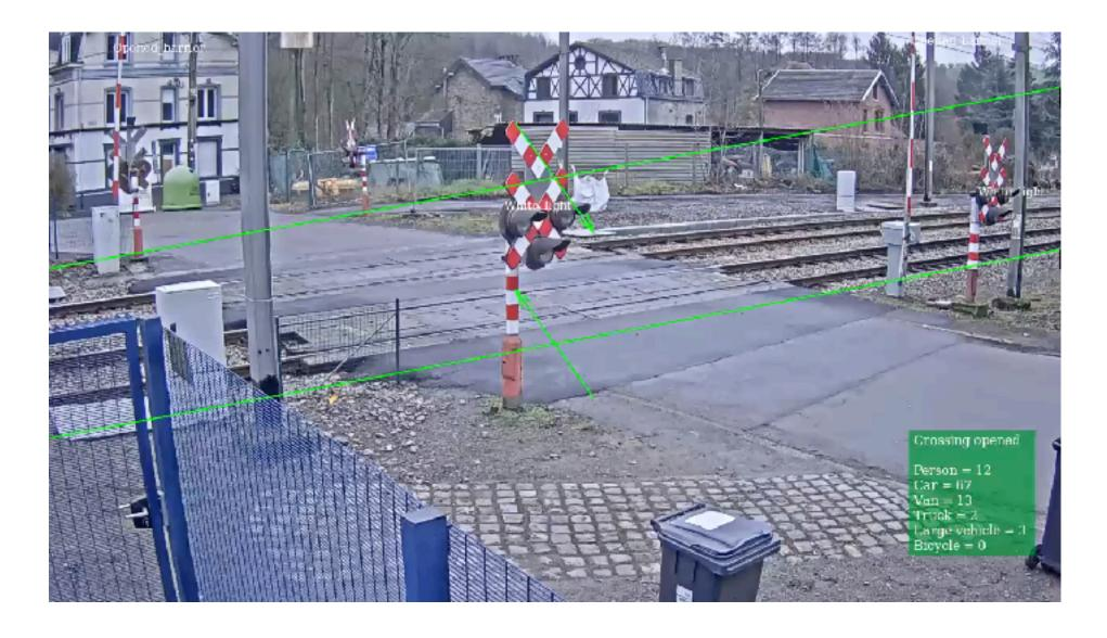
Green lines : automatic danger zone detection In the green box at right bottom : counting and crossing phases
