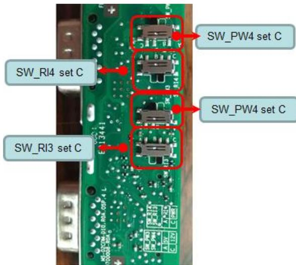
Power 12V setting: Change at C location from SW\_RI3 and SW\_RI4 and at C location from SW\_PW3 and SW\_PW4
