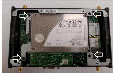
2. Loosen 4 screws as the arrow directions.
