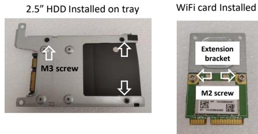
5. HDD tray & WiFi card installation. (Screws & mPCIe extension bracket are in accessories kit . )
