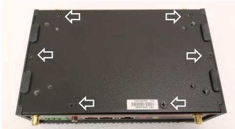
1. Loosen 6 screws from Bottom cover as the arrow locations.
