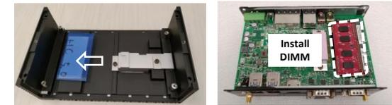
9. Remove the film from top cover & install DIMM to MB.
