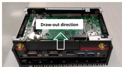
8. Draw the MB sub-assembly out from top cover as arrow direction.
