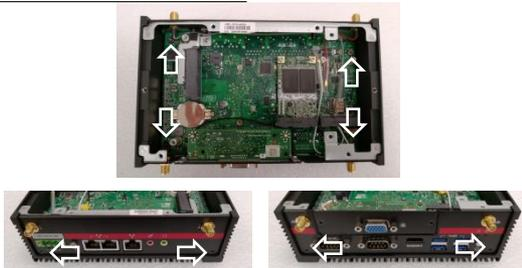
7. Loosen 4 screws from MB (2 screws from front & rear cover).
