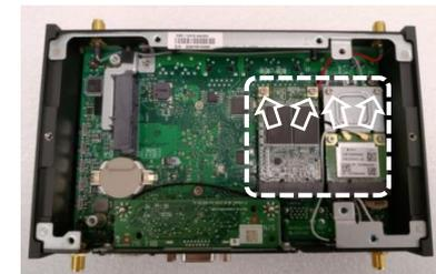
6. Install SSD or WiFi card Mini PCIe slot & plug in antenna IPEX header on WiFi card (White cable for Main & black cable for Aux location).
