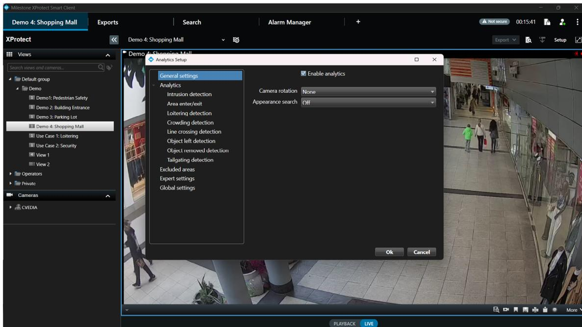
Check the “Enable analytics” box to activate the analytics on a given stream.
