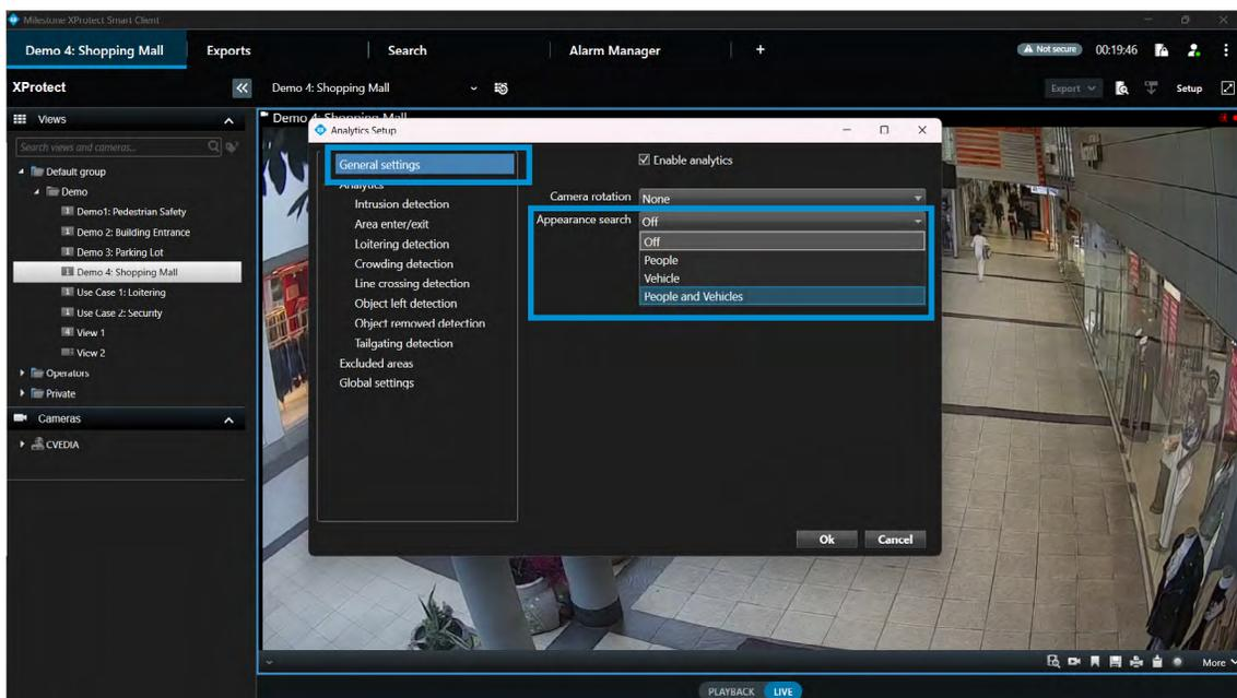
Once the Appearance Search feature is enabled, you can leverage Smart events functionality to filter out objects within existing detections based on vehicle type/color and clothing color.
