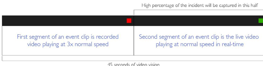
Operators watch the short clips displayed to determine what, if any, action should be taken. Each video clip is displayed for approximately 20 seconds up to the default maximum of 45 seconds before disappearing automatically. This period ensures that there is footage for operators to obtain sufficient context for investigation before displaying the next anomaly.
