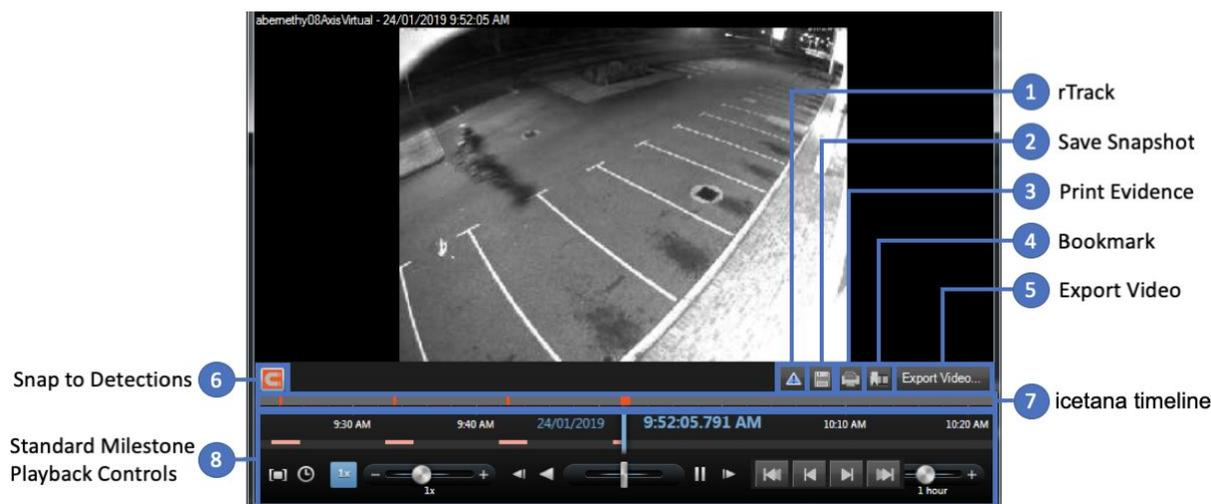
Figure 10: icetana Playback floating window controls
