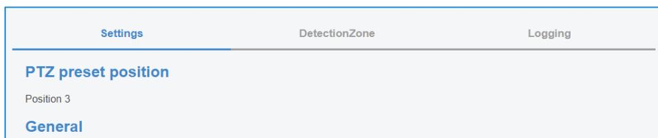
**! Notice:** Make sure all relevant PTZ positions are properly configured and named. Even for a camera with motorized lens that remains in fixed position after initial configuration, this position should be named (e.g. 'home'). Unnamed positions will not be identified, and the algorithm will not start.
