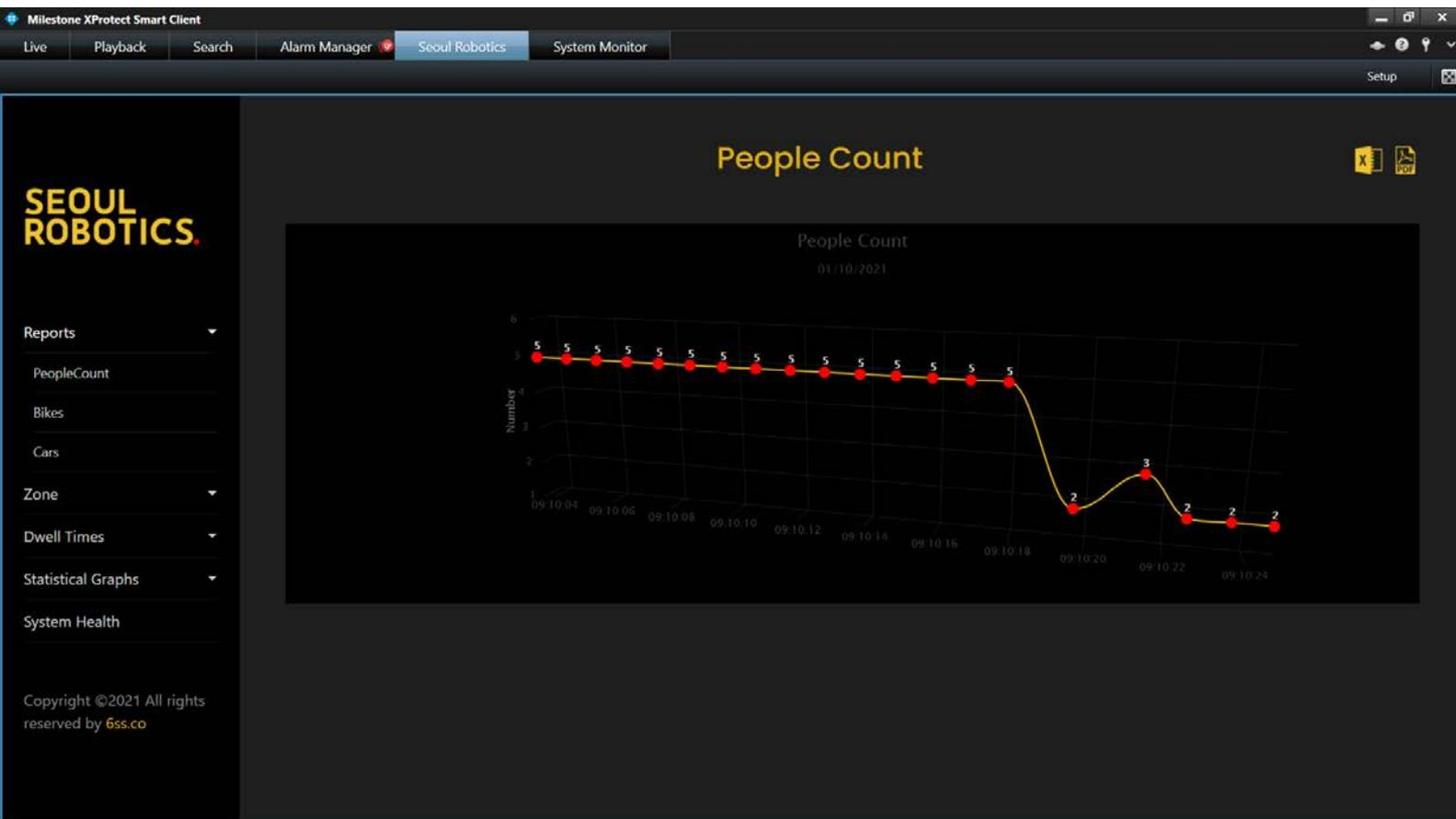
In the Object Count per zone, the user can check the number of detected objects that entered each event zone (for example 200 objects entered the zone 1005).
