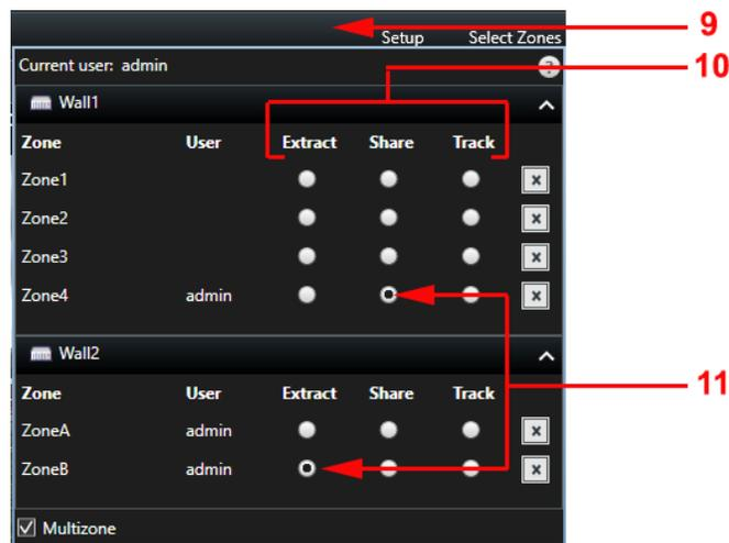
When Multizone is selected the methods of display are removed from the Workspace Toolbar (9) and incorporated into the Multizone dialogue (10). This enables a View or View Item to be displayed on multiple zones and walls using different display methods. In the example above, the View or View Item has been Shared to Zone 4 on Wall 1 and Extracted to Zone B on Wall 2 (11).
