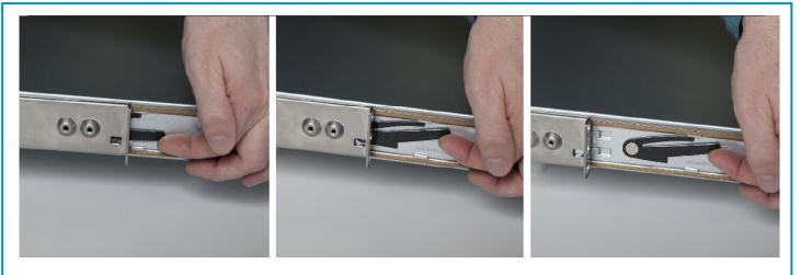
Slide the machine out until it stops, then pull the release mechanism as shown above to complete removal.
