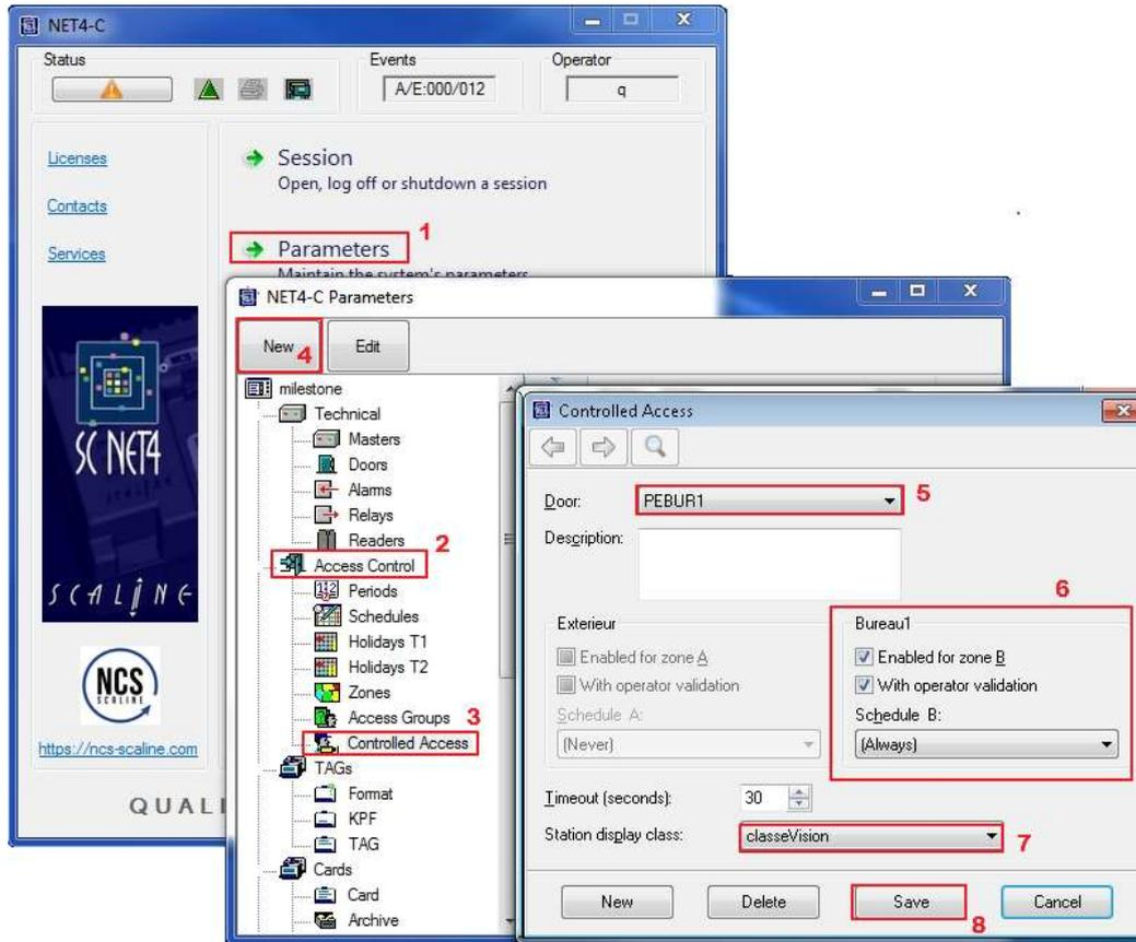
Figure 8: Controlled access setup to enable management from Milestone XProtect Smart Client.
