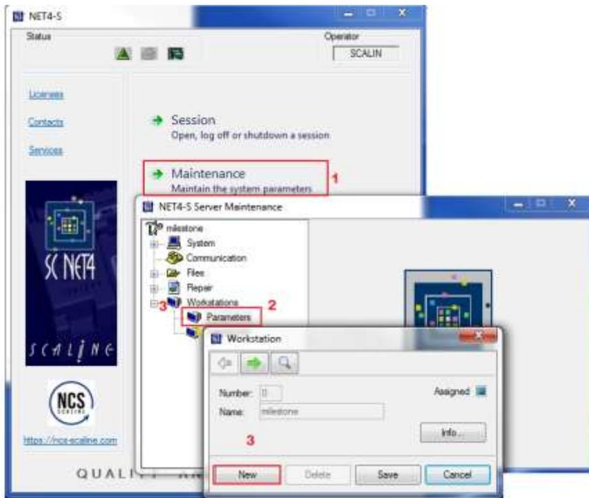
Figure 5: Creating a dedicated client station for the XPPLUG plugin instance.
