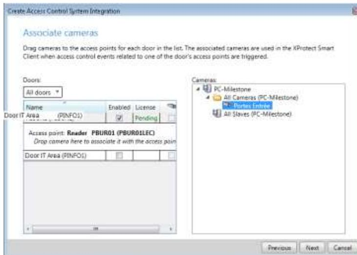
Figure 21: Association of cameras with doors/ access points of the XProtect Access Control plugin.
