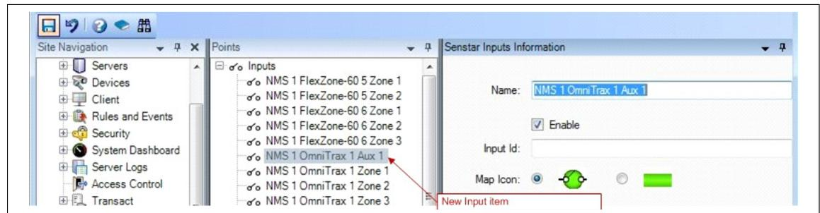
Figure 21 Manually adding an input
