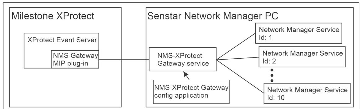
Figure 1 NMS-XProtect integration block diagram
