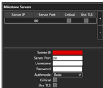
On larger Milestone systems that include additional servers for either load or redundancy, or both, it may be necessary to add these servers to the configuration. The primary server should always be added in the main part of the configuration and only additional recording and events servers should be added here. To add additional servers:
