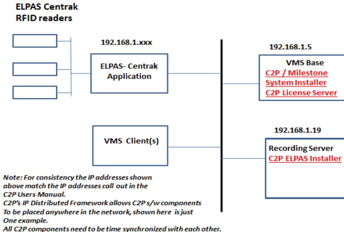
Figure 1 below depicts a typical C2P ELPAS CENTRAK deployment topology.
