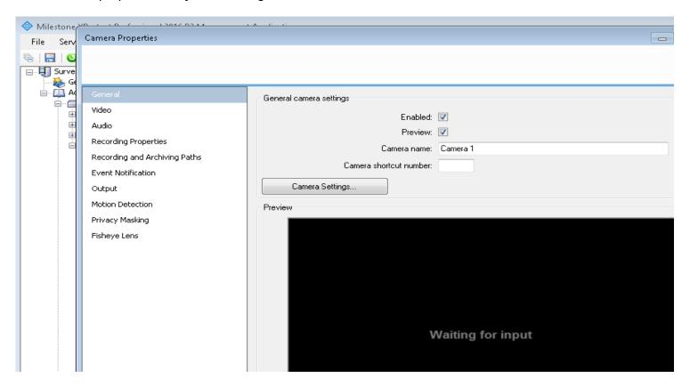
Configure Camera properties as shown below. Assign the getportX URL connection for each ATM / Teller Workstation data sourcing point where X is the virtual camera differentiator. If you have 20 ATM / Teller Workstation detection points you will have getport1 thru getport20 virtual cameras.
