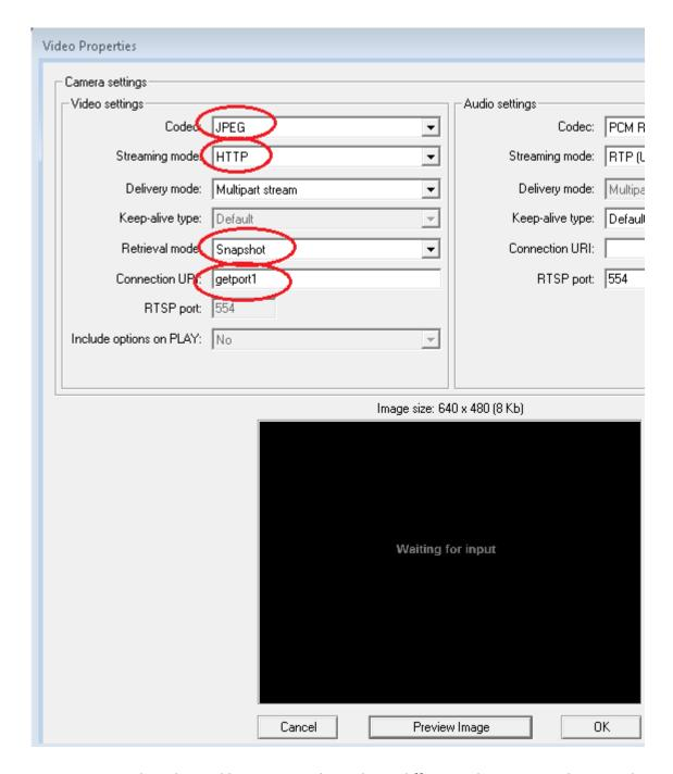
**Note**: Retrieval mode used here is Snapshot, this is different when using Milestone Plus Series mode.
