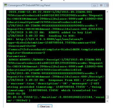
The screen below shows activity in the C2P ESE when data is being received from the C2P ATM and Teller Workstation integration.
