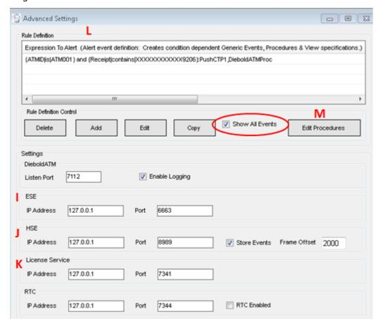
**I** = Event Streaming Engine (ESE). The ESE is normally installed on a recording server associated the ATM / TELLER WORKSTATION video. See also <u>Figure 1</u>
