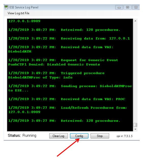
The "Config" button on the bottom of the ESE control panel brings up some configuration settings for the ESE. For non-demo installations the one setting that will likely need to change is the Generic Event IP address.
