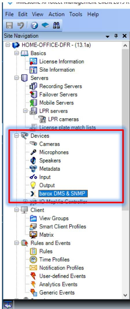
After the installation you can start your XProtect Management Application. After the first start you will find a new Entry under “Devices” called “barox DMS & SNMP”.
