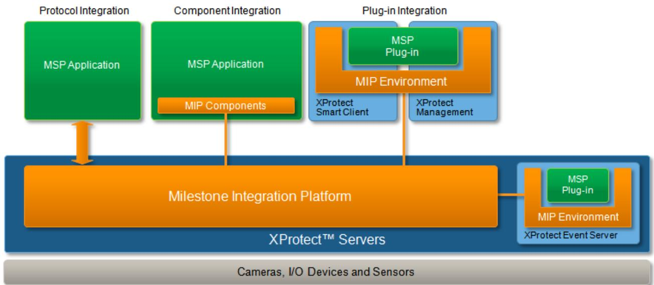
The integration consists of a MIP Plug-in for the Milestone VMS. It is installed on the Server side for the configuration and retrieval of events and is running inside the Milestone Event Server.
