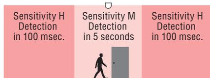
A specific detection zone, such as a door or window can be set at a different sensitivity level.
