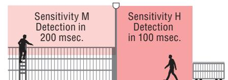
The sensitivity can be adjusted to the assessed risk per zone: high sensitivity to detect a running person and medium for a climbing intruder for instance.
