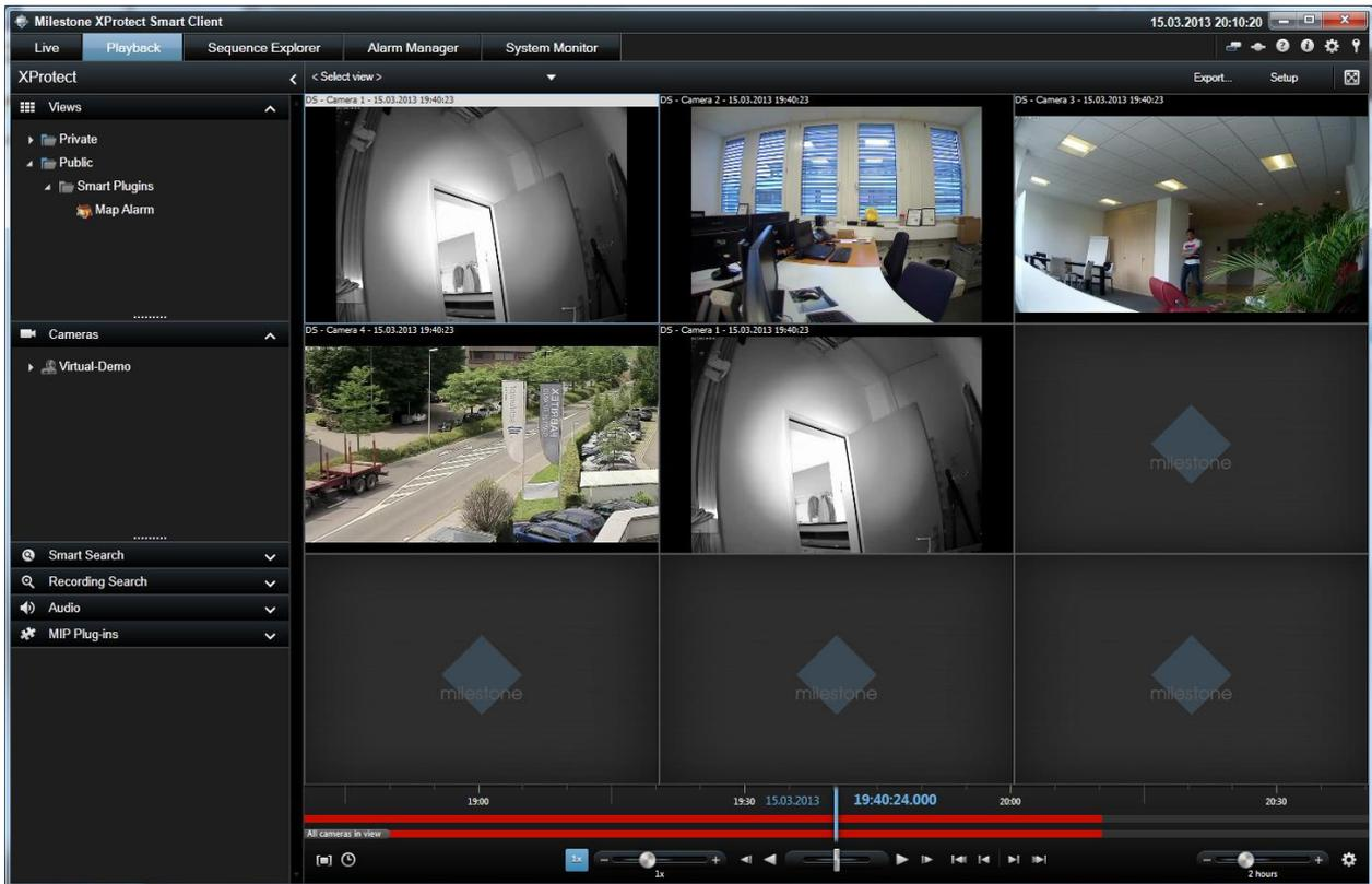
Smart Alarm switches automatically to the Browse Mode and creates a view, which contains all related alarm cameras.
