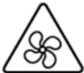
This symbol indicates the presence of a moving fan blade. If the spinning blades are contacted, the potential for injury exists.
