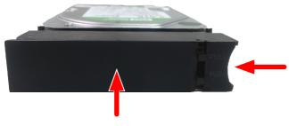
Push in the center to insert the drive carrier into an empty drive bay.
