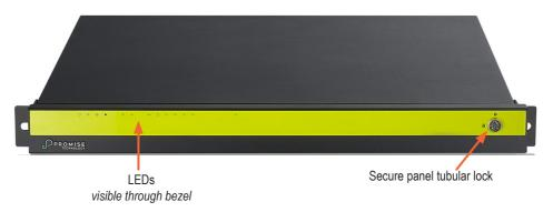
The Vess A3120 is shipped with a lockable front secure cover which must be removed in order to access the hard disk drive carriers. Use the tubular key to lock or unlock this cover.
