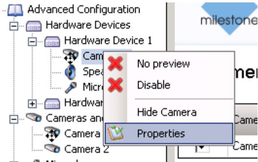
From the properties menu select Output. Ensure that the output is associated with the camera (Highlighted in blue). **Ensure that the output device is also contained in the manual activation section (highlighted in red).**
