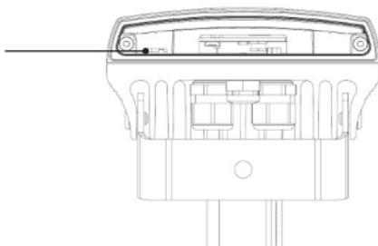
Baseplate fixing screws: Torque 0.6Nm
