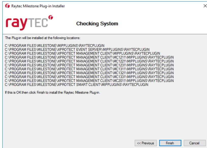
**Please note that it will be necessary to restart the XProtect server once installation is complete, the event server must be restarted in order for it to recognise that the Raytec Milestone Plug-in is available.**
