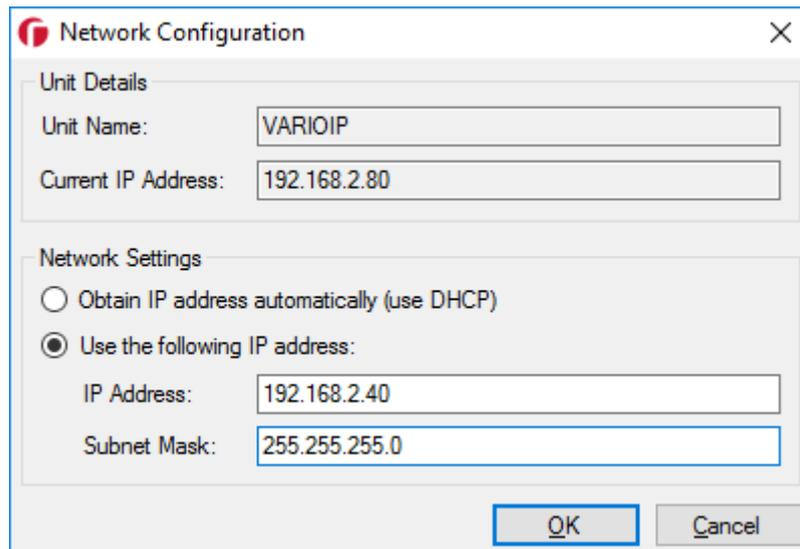
After inputting your changes click save and you will be notified that this action will cause the illuminator to temporarily lose communications while it reconfigures itself. You will then be back at the main window of the Discovery Application. After around 30 seconds you should be able to click the *Discover* button again and the illuminator will reappear in the list with the settings that you changed.
