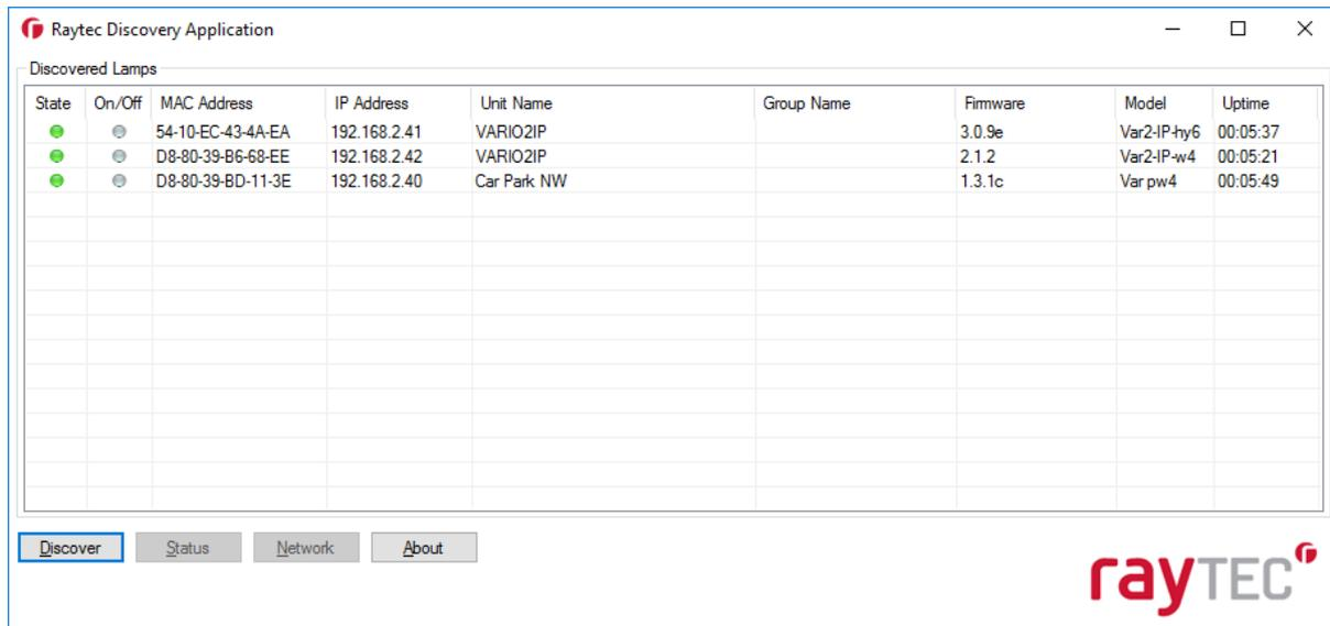
Note that any illuminators you wish to control through your VMS system should be configured for VMS control. This can be done through the illuminator's web interface on the *Settings/Groups* page. Double click on the individual illuminators within the Discovery Application to access the illuminator's web interface.
