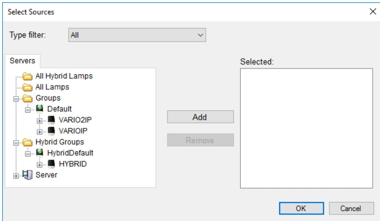
Just as they are in the tree in XProtect, the illuminators are shown under *Group* if they are standard, single wavelength illuminators and *Hybrid Groups* if they are hybrid illuminators. You can have as many lamps as you wish triggering the alarm you are creating.
