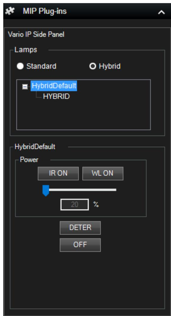
The actions available through the Smart Client are timed. Standard illumination will time out after 5 minutes and deterrent will trigger the Hi-Lo pattern at a fast speed for 30 seconds, in both cases, the illuminators will revert to their previous states on time out.
