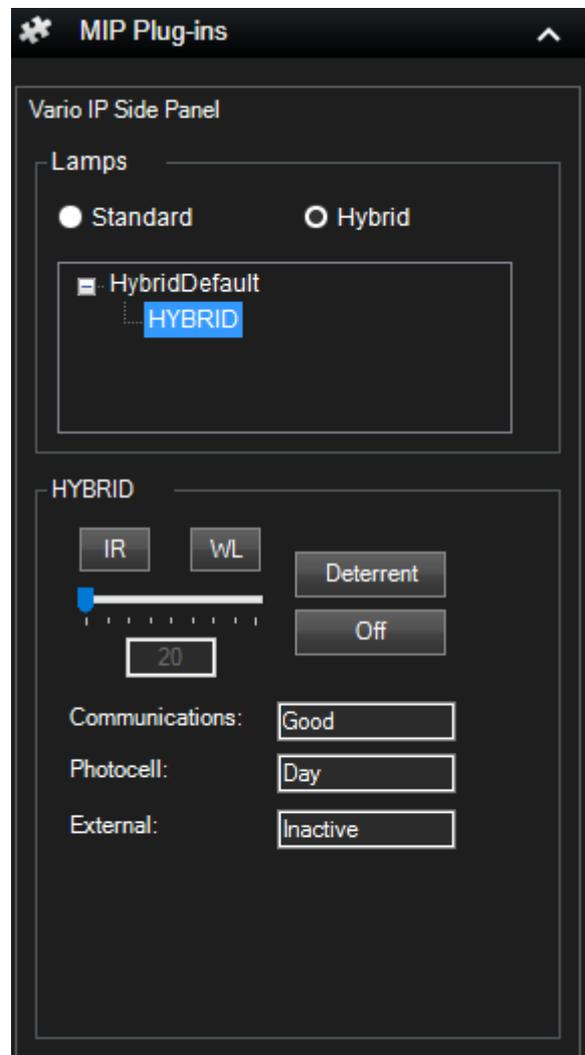
The On and Off (standard single wavelength illuminators) and IR and WL (hybrid illuminators) indicators show the current status of the illuminator. You may select either On or Off or IR or WL to change this status. When the illuminator is on you may move the power bar to change the power intensity of the selected illuminator. Any change to the illuminator on status or power level will remain valid for 5 minutes.
