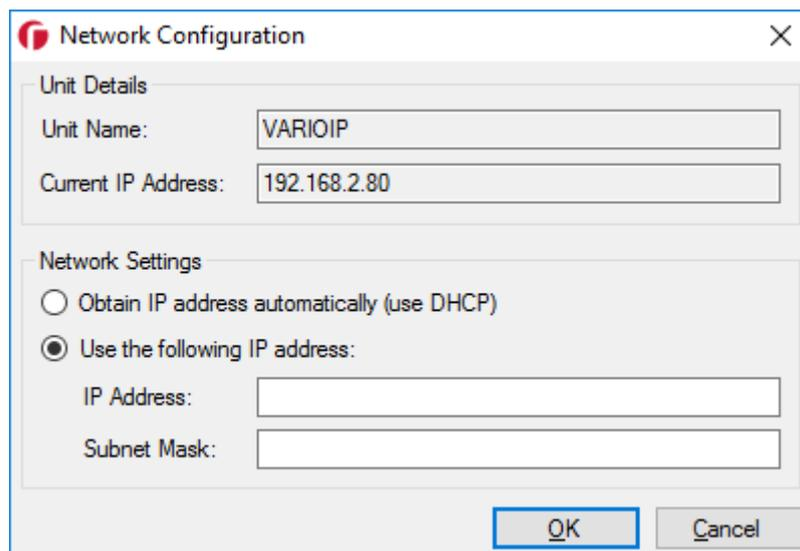
You can choose to enable DHCP here should you wish. This will make the illuminator request an IP address from the DHCP server on your network, however this method does not guarantee that the IP address of the device will remain the same throughout its lifetime on the network.
