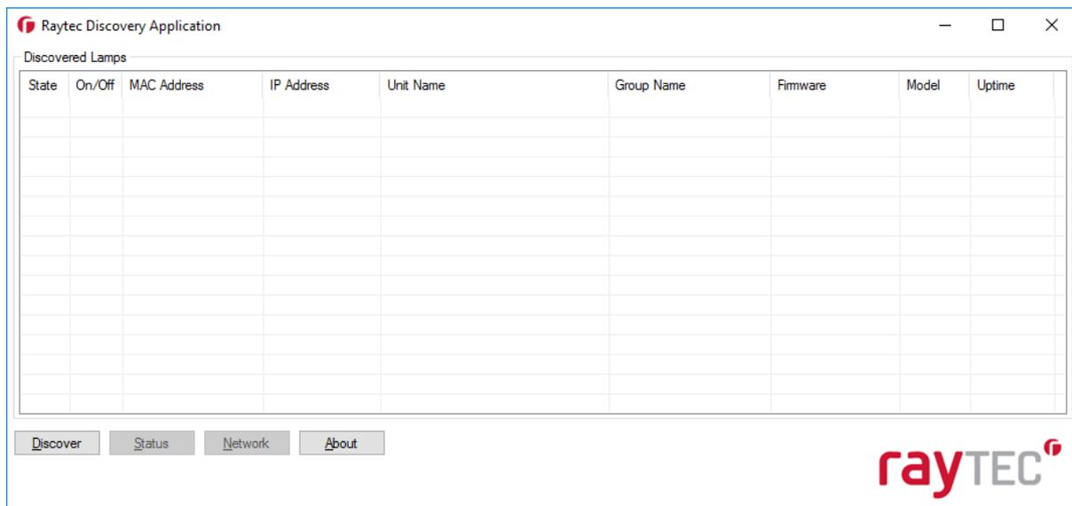
Click the *Discover* button and any Raytec network illuminators that are on the network should appear in the list.
