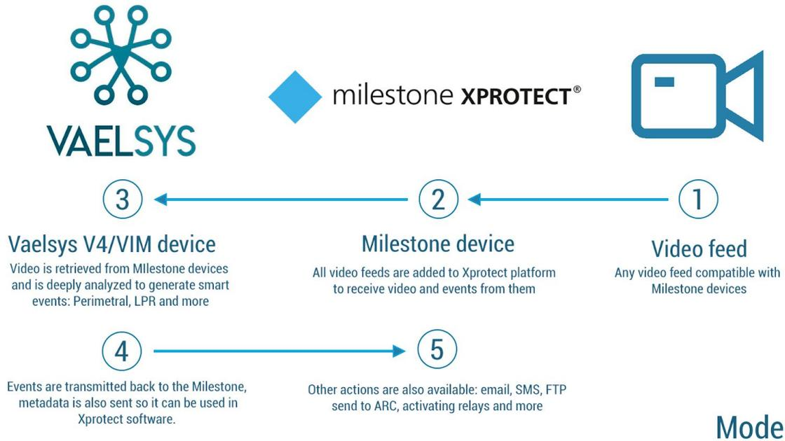
All cameras are added to the Milestone device. Then, the video stream of each video source is streamed again to Vaelsys analytics device where is processed. Events are sent back to the Milestone device so can be managed as desired back in Milestone services.
