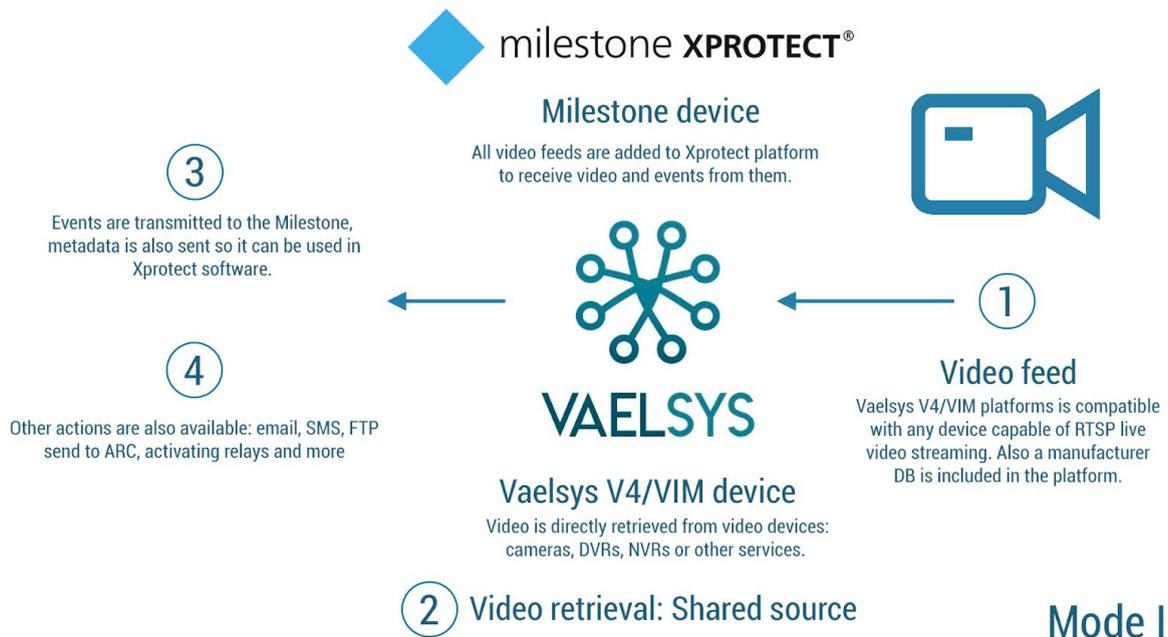
In this case, both the Milestone device and the Vaelsys analytics device gather video directly from video devices. Using this method has some advantages:
