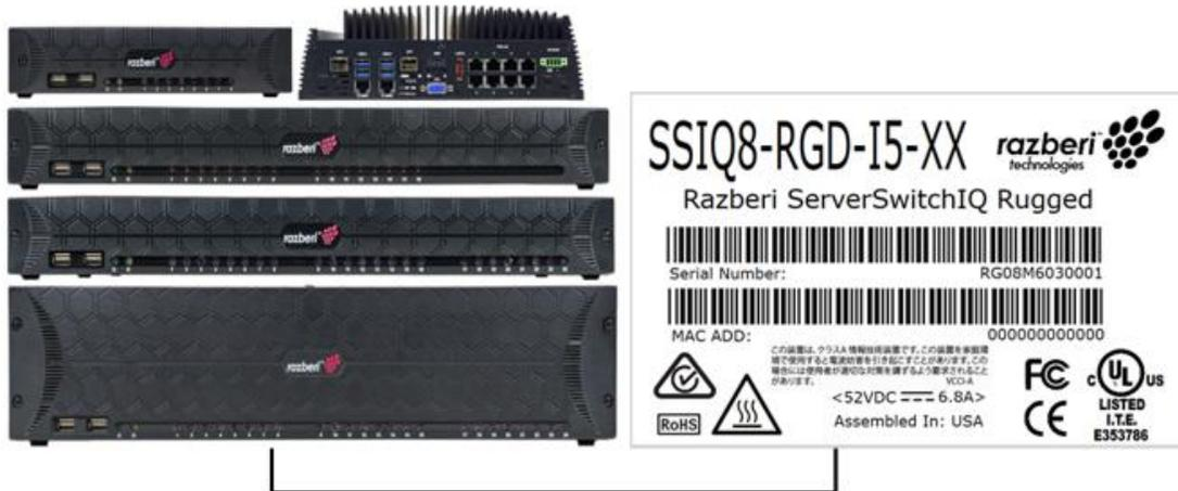
Located at the bottom of every SSIQ appliance is serial / model label detailing all the information needed to identify SSIQ model.
