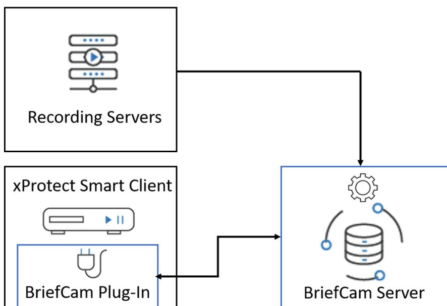
The BriefCam UI appears in a “Video Synopsis” tab in the xProtect Smart Client. The user can use the entire BriefCam user-facing UI inside the client. Once a video needs to be fetched from the VMS the BriefCam server interfaces with the Milestone Recording Servers (through the MIPS SDK) and fetches the required on-demand or real-time video. BriefCam processes the video and presents the results to the user within the xProtect Client.
