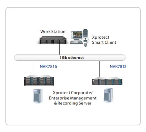
The specific configurations detailed above were chosen in order to conform to the recommended Milestone storage configuration; providing a live database and an archive database for each recording server.
