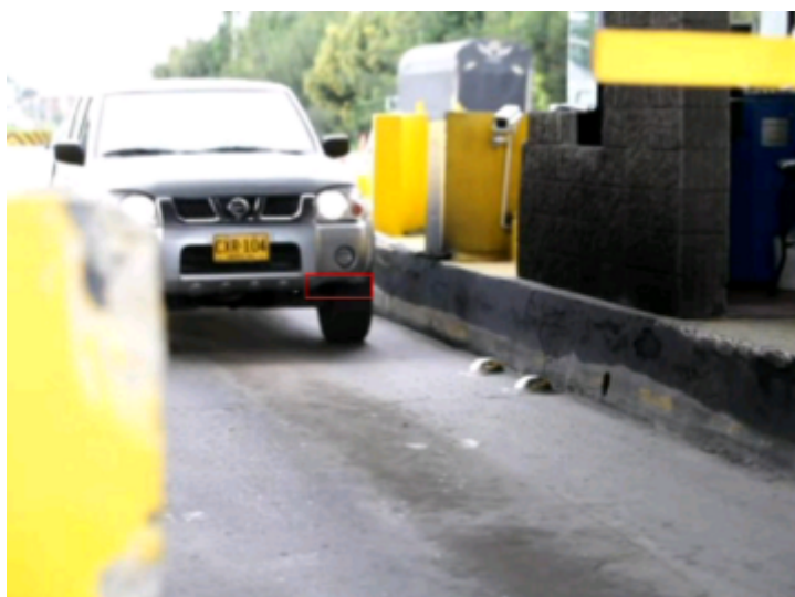
Figure 11: An example of an image where the license plate frame does not cover the license plate
