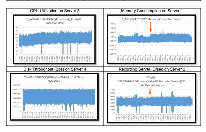
There were a couple of changes to the video stream profile between scenario 1 and scenario 2. The stream size of each individual camera was increased from 1.90 to 2.09 Mbps. This affected the total disk throughput by increasing the amount of data being recorded from 59 to 65 MBps on each server. With increased data, we also saw an increase in CPU consumption and an increase in IOps.
