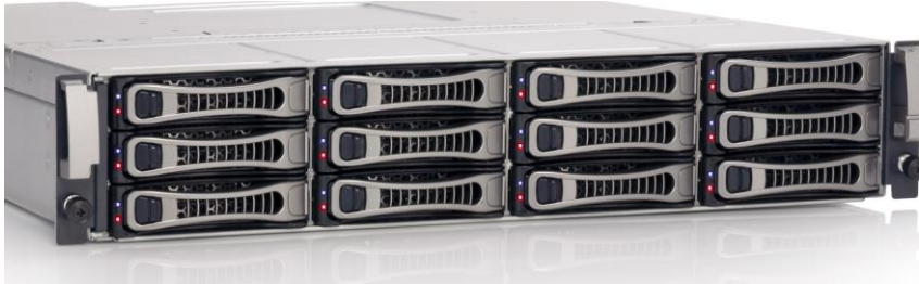
Figure 3-11 HDD Assembly installed in Chassis
