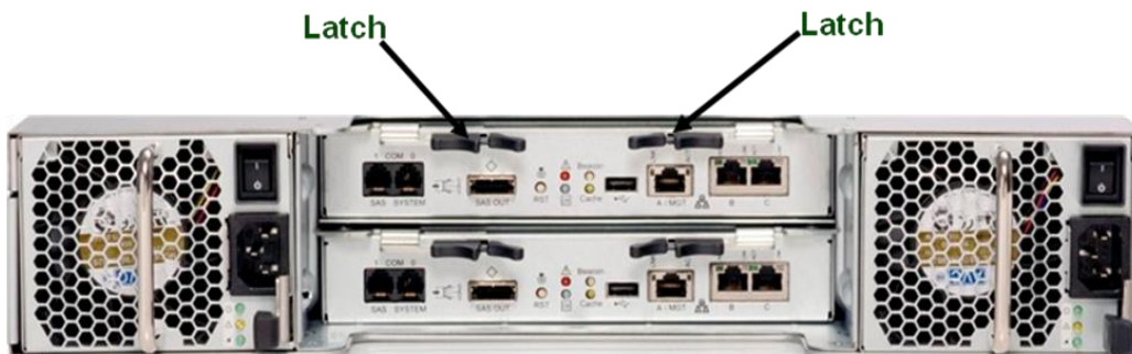
Figure 3-5 Inserting the Controller Module
