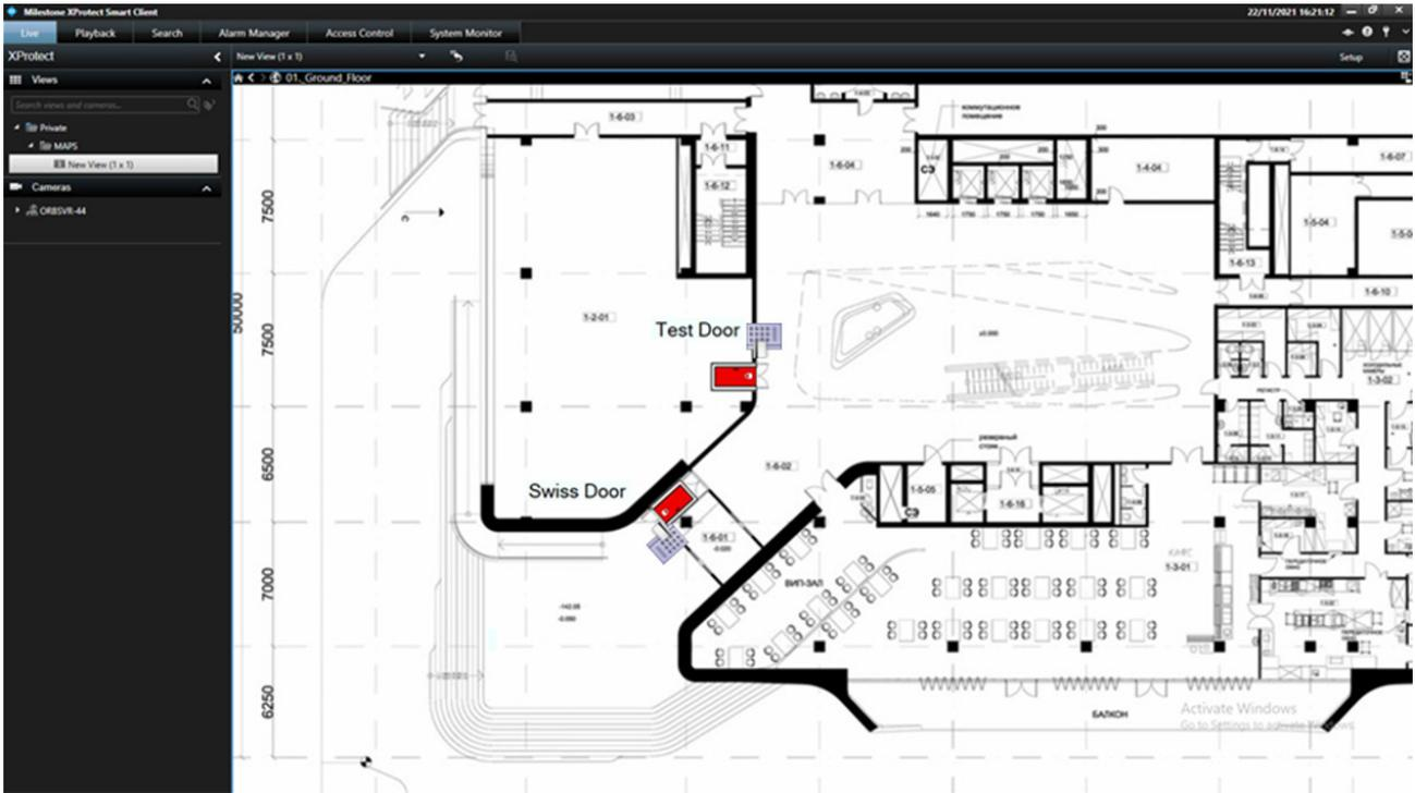
Doors will show Red when locked, an Open door when unlocked. For the override states these show with bars on the door to indicate a fixed state of Locked (Red) or Unlocked Green). Readers will flash green or red depending on the badge presented and be in the normal state otherwise.
