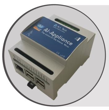
AI-Appliance is the plug and play embedded solution powered by A.I. Tech, provided as an integrated hw+sw solution; all the video analytics sw is already preinstalled in the box, provided with a 4-modules wide DIN case [71x62x90mm].
