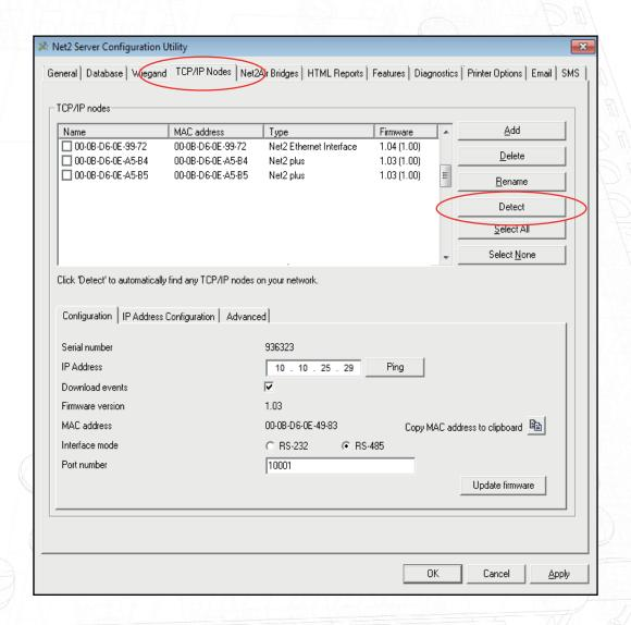
ensure that the same IP address is issued each time, should the unit be reset. Consult your network administrator on detail of how to reserve IP addresses. The unit's MAC address can be read from inside the plastic enclosure, and will be required by the Network administrator to enter the reservation.
