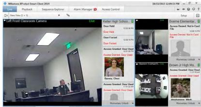
The Access Control tab provides a dedicated view for all the DNA Fusion access control events along with the cardholder information and photo if available. The door view includes a list of the doors and their current state. When an event or door is selected, all the associated cameras show the event or live video on the right-hand side of the screen together with detailed cardholder information.
