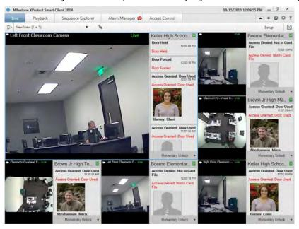
When an Event is selected from the list, the live video automatically pauses and changes to independent playback of the event video. To go back to viewing live video, either **click** the event again or **click** the Independent playback icon on the camera toolbar. If the system and the event hold cardholder information, **click** the Search icon next to the cardholder name on a selected event to jump to the Access Control tab and view all events associated with the cardholder.
