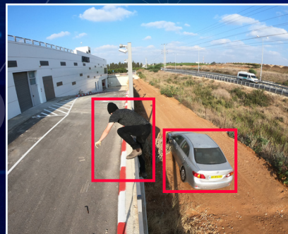
Real-time detection (rule-based) of a stopped vehicle in sterile zone and perimeter breach
