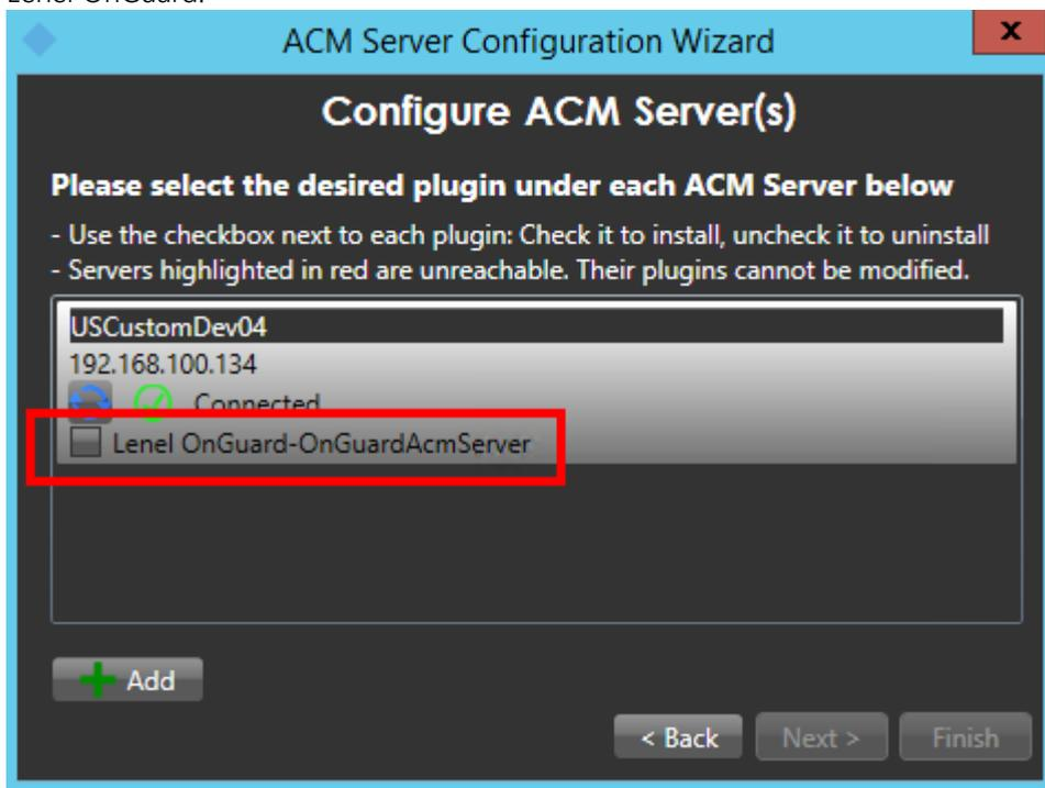
Check the box marked below and press next to install a MIP plugin on this host to connect to the Lenel OnGuard server identified.
