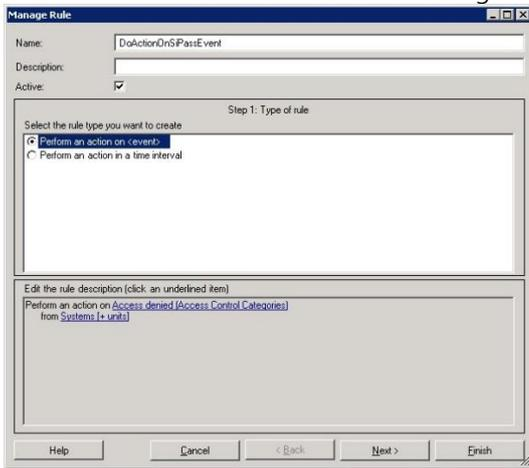
Press next and select the optional time frame when the action will take place. In this example no time frame has been selected, this means it will always execute.
