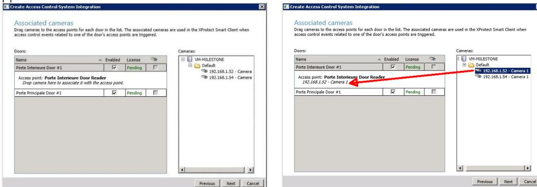
When there is more than one access point per door, you can select the different cameras for the different angles. You can also select more than one camera per access point:
