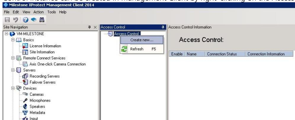
This will pop up a wizard to step you through the access control instance creation process. Type a name for the instance of the plugin you wish to create and select from the drop-down box the integration plug-in. Note that you will find a plugin named Lenel-OnGuardAcmServer-`{ServerName}` where `{ServerName}` is the name of the machine where Lenel OnGuard and ACM Server are installed.
