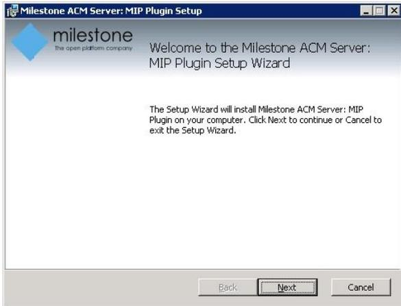
The installer will detect the presence of the XProtect Event Server on the machine and will refuse to install if it cannot be found. It is recommended to leave the default install path as displayed below and press next.
