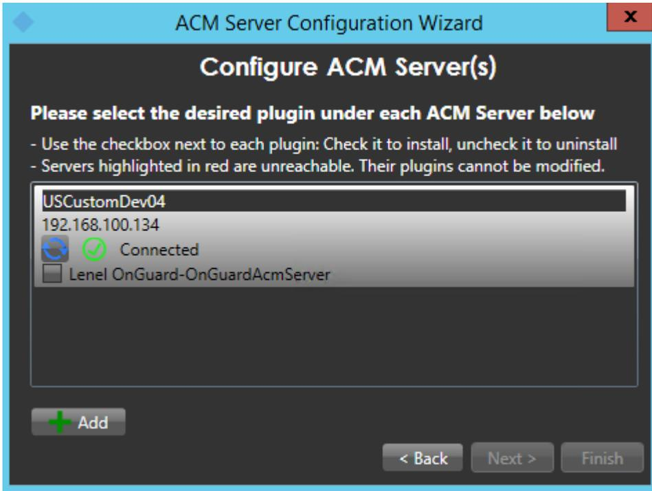
Note that the most common causes of the wizard not being able to connect to the provided server is that 1) you entered the wrong IP information, or 2) the ACM Server on the Lenel OnGuard machine is not running with sufficient administrative privileges.
