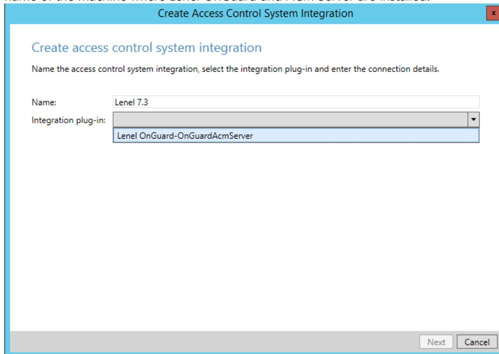
After selecting the plugin, you will have to provide credentials and parameters to configure the connection to the Lenel OnGuard database server, optimize particular settings, etc.
