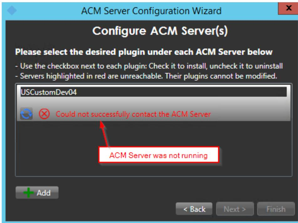
Once you have a successful connection, notice that there is a list of checkboxes under the server heading that represents all detected ACM server plugins installed on that machine. In this case we are looking for Lenel OnGuard.
