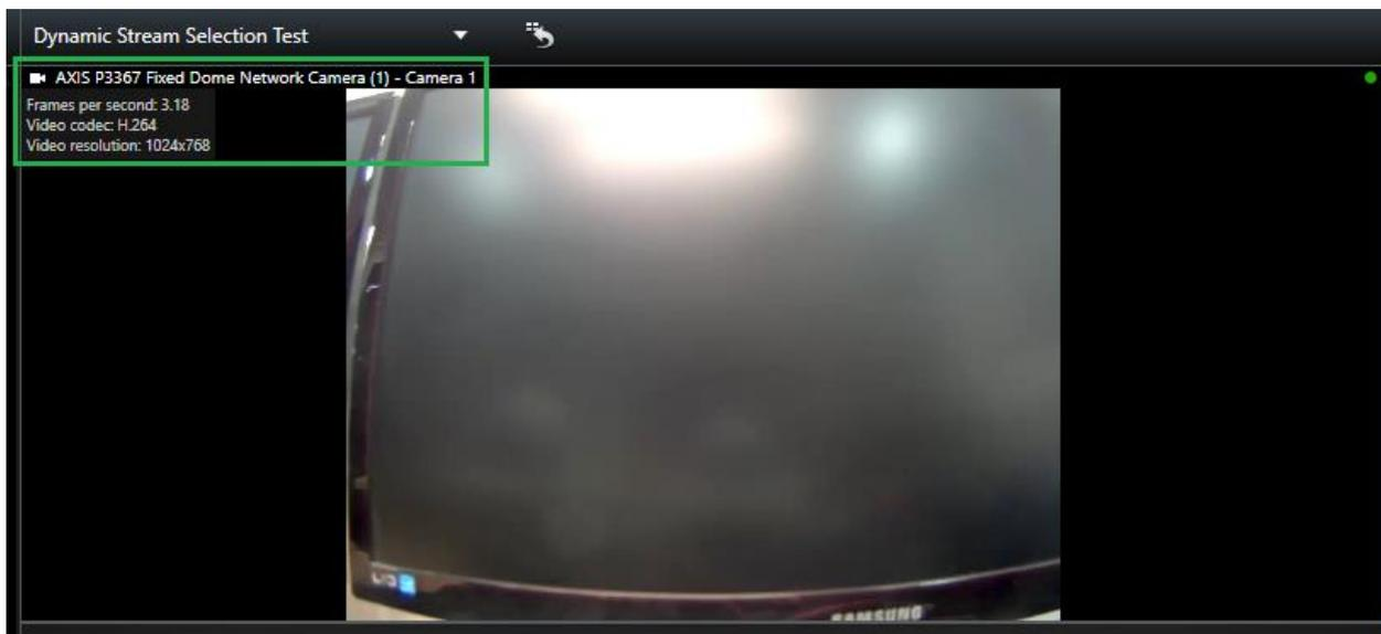
When **AXIS P3367 Fixed Dome Network Camera (1) - Camera 1** view reaches the size 800x600, the stream will be switched to **High** as shown below on the figure.
