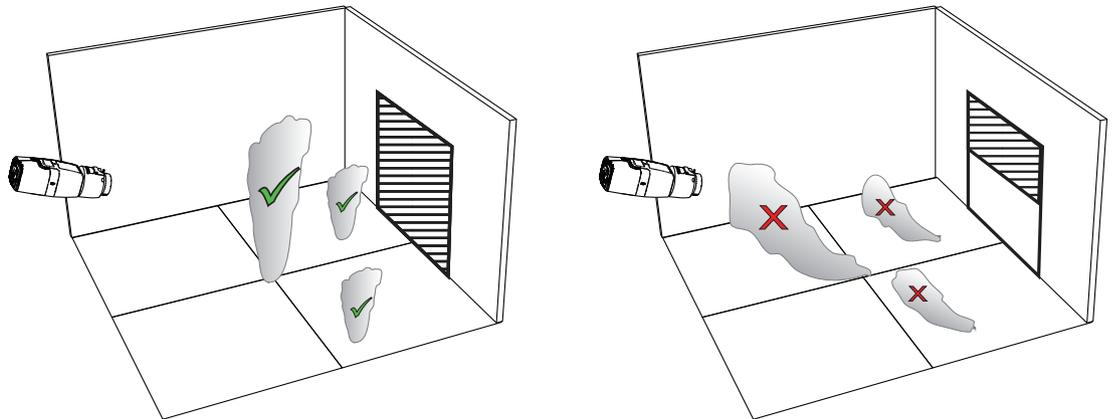
The intelligent smoke detection covers a large area of application. Nevertheless, there might be some disruptive factors in the operational environment of the customer. Objects with a similar movement pattern of smoke might cause false alarms, e.g. escalators or conveyor belts.
