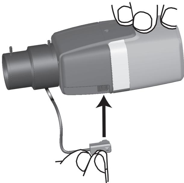
Plug the lens connector into the camera (it automatically detects the type of lens).
