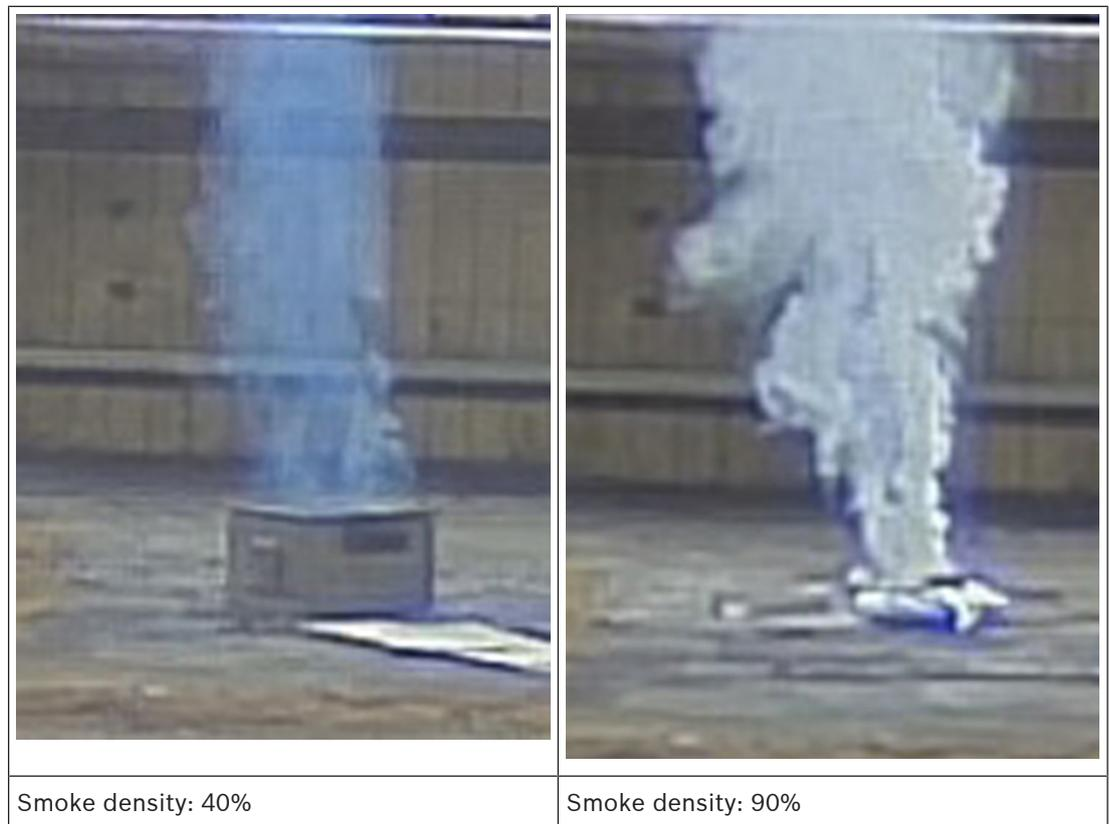
In regular conditions with an equal colored background, smoke is visible when the smoke density exceeds 40%.
