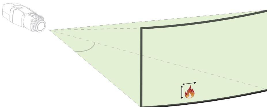
The monitoring area defines the effective space that can be observed by the video-based fire detection. It is depending on the setting of the camera lens.
