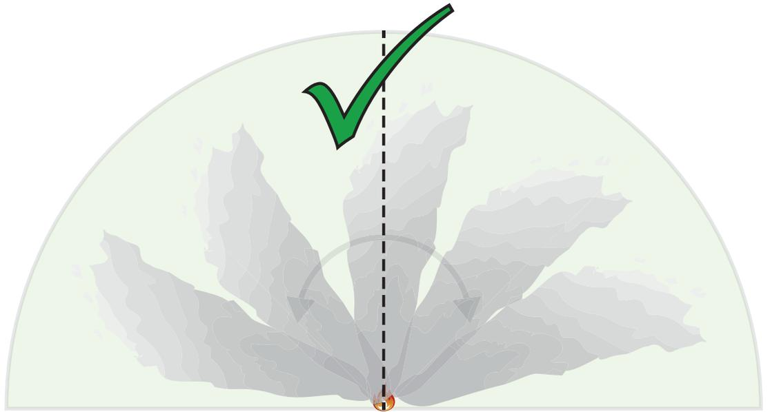
Smoke plumes must move in a constant direction with a minimum density to be detected by the video-based fire detection. Irregular expanding smoke and smoke plumes moving in the direction of the camera might not be detected.
