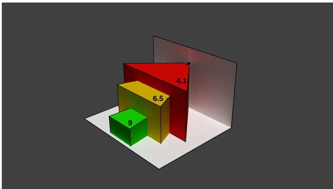
The maximum width of the field of view may be realized by the minimum focal length. This adversely affects the maximum distance to a detectable fire (red).
