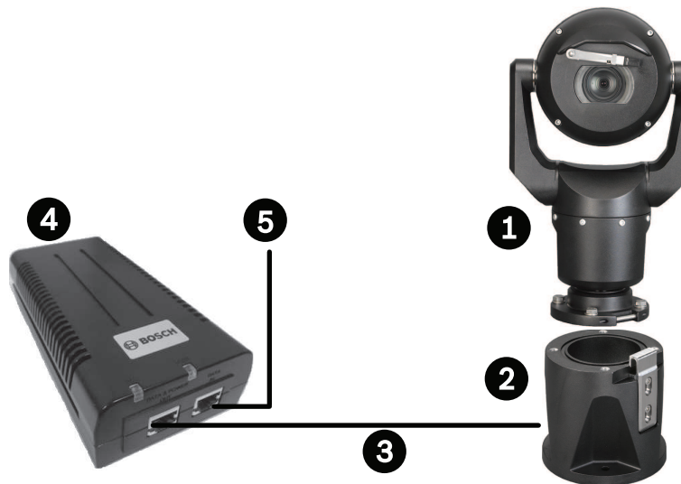
Figure 9.1: Typical IP configuration with High PoE Midspan (no I/O connections)
