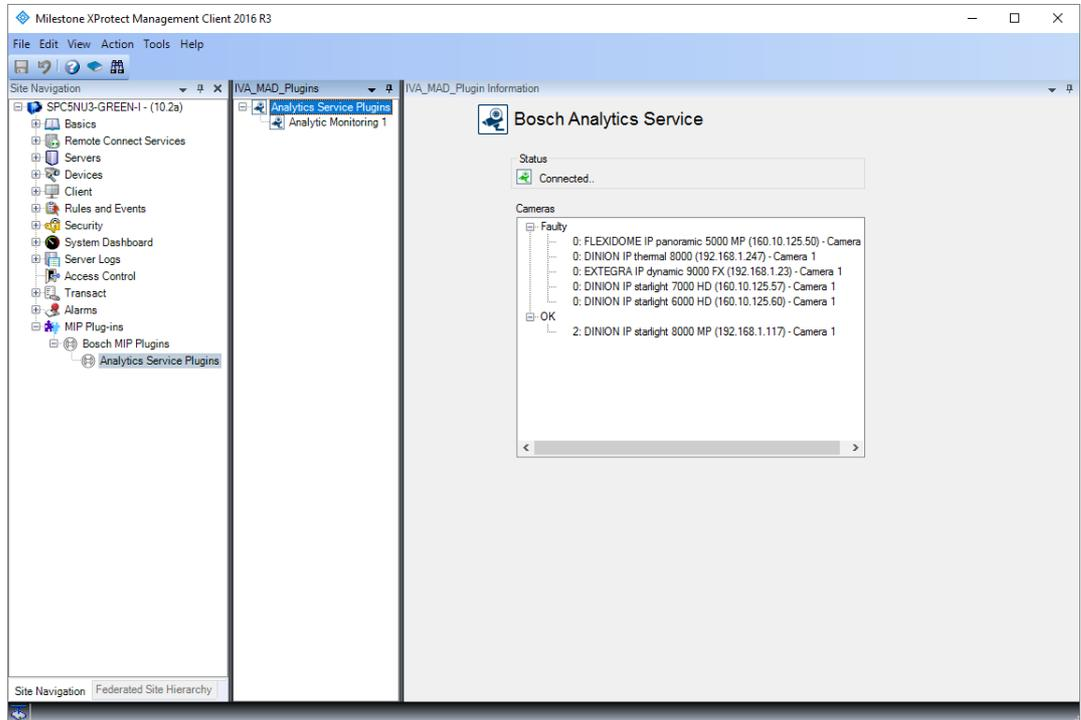
The monitoring page shows cameras with an error in the **Faulty** section and cameras that are working properly in the **OK** section. The camera name is preceded by the number of generated events, as depicted above.
