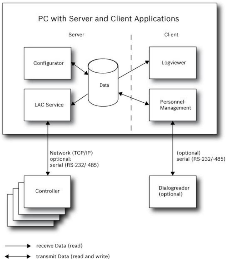
**Figure 1.1: System Overview – Single Computer Configuration**
